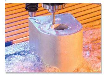
Cut **ANY** material up to 200mm thick Bed-size of 4 x 2m Accuracy of + / - 0.1mm Tolerances as close as + / - 0.005" No Heat Affected Zone (HAZ) **Learn more:** www.wecjet.com
